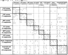
Figure 1: A DSM of a commercial jet engine (From: Sosa et al., 2003)
