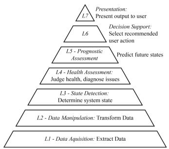
Fig. 1. OSA-CBM Framework, adapted from [44], [79], [80], showing the seven levels required for an effective IVHM system.
